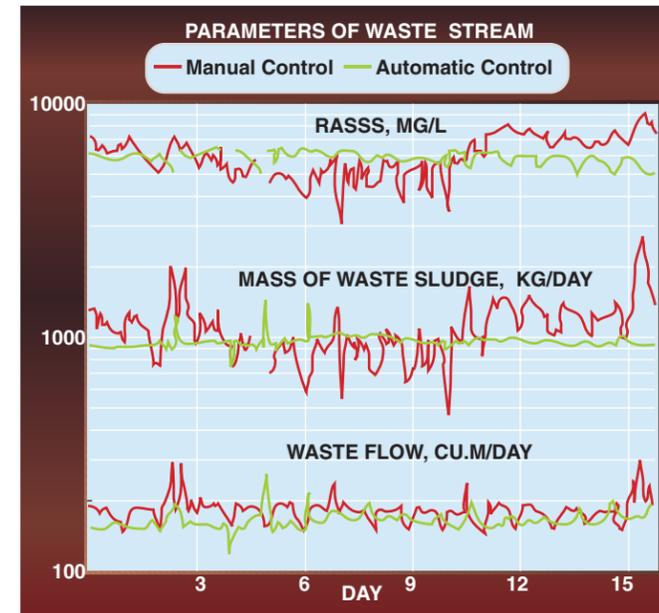
SRTMASTER maintains constant mass solids loading to activated sludge thickeners. As a result, thickener performance improves considerably.
