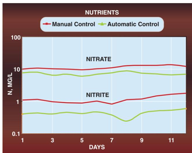
Under constant SRT, nutrient removal is improved because ammonia removing autotrophs and denitrifying heterotrophs function under optimum conditions.
