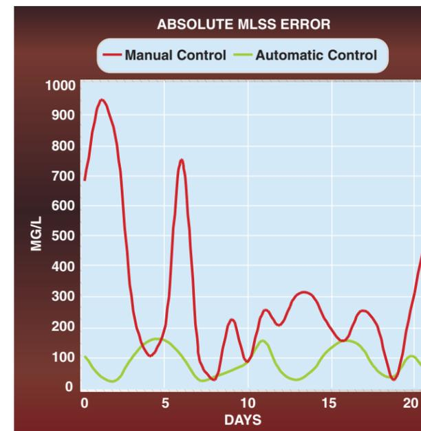
Suspended solids concentration has less variability due to SRTMASTER's ability to measure TSS and calculate wastage on-line. As a result, clarification is improved, especially during peak and storm flow conditions because solids mass loading on clarifiers is reduced.
